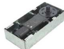
FLS-25 Speedy head Size: 28.3*13*6.5cm Degrees: 90 Degrees Positioning Max door weight: 90kg
