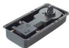
FLS-28 Dorma head Size: 270*130*50mm Degree: 90 Degrees Positioning Max door weight: 90kg
